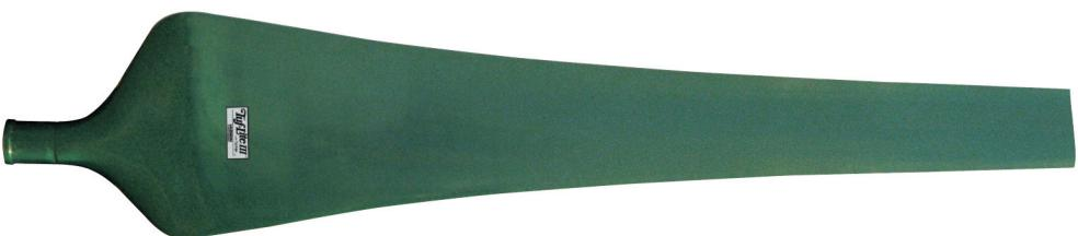
Tuf-Lite III™ is a refined and enhanced one-piece blade constructed from fiberglass reinforced vinyl ester resin coupled with leading and trailing edge protection, and superior "UV" protection. Developed from the most severe strength-testing program to date, Tuf-Lite III® blades are individually balanced, interchangeable and will install in HUDSON hub designs. Initial size are from 28 feet to 10 meters in diameter.
